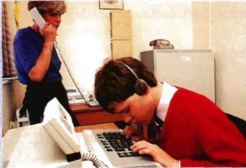
A blind student using an adapted keyboard, in the presence of his tutor. The headphones and a screen reading program allow him to hear the text from the screen.
