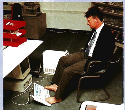
Bob Love was born with no arms. He uses an overlay keyboard with his feet and the computer and monitor on the floor. The key overlays give a much larger surface for each key.
